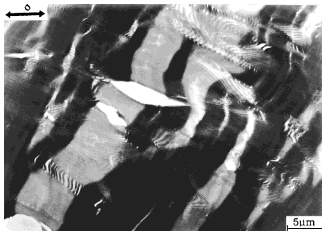
Figure 15. HVEM micrograph of deformation zones of an intermediately segregated PS- b -PBMA diblock copolymer at \chi N = 39 (SBM315, \Phi_{PS} = 0.70 , M_n = 315 kg/mol, lamellae). The craze propagation is influenced by morphology and does not occur perpendicular to the external stress direction in all cases.
